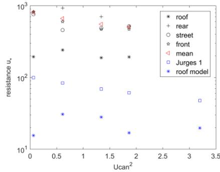
Figure 5.  $Res_{facet}$  averaged over different facets as a function of  $U_{can}^2$ . The mean of  $Res_{facet}$  is the average over rear, ground and front surfaces. From low to high  $U_{can}^2$  corresponds to  $H/W = 2, 1/5, 1/11, 1$  and  $1/2$  respectively.
